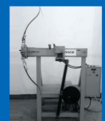
Dry fire testing for breaking and strength of limbs
