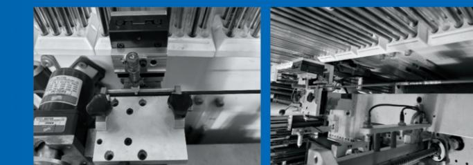
After installing on the cushion plunger test equipment, measurements of the friction were taken 3 times for each material, repeated 2,000 times. Measurements of the abrasion of the arrow surface and abrasion of the pressure point per number of time were also collected.
